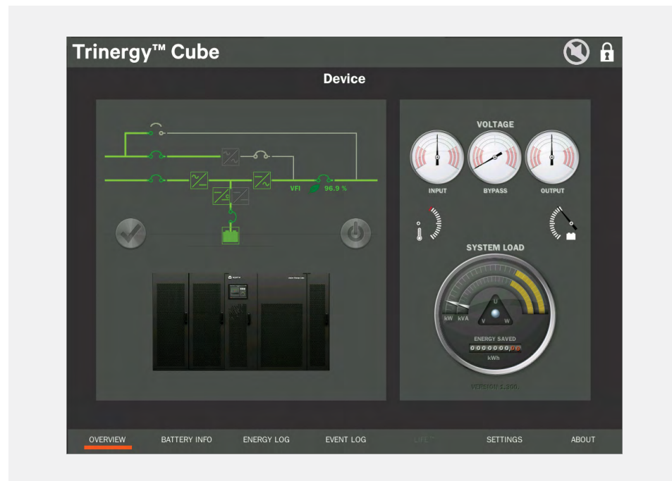
Liebert® Trinergy™ Cube LCD touch screen: interface for data tracking, logging and event analysis
