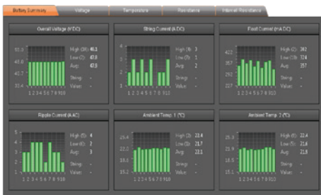
View data on parallel battery strings simultaneously
